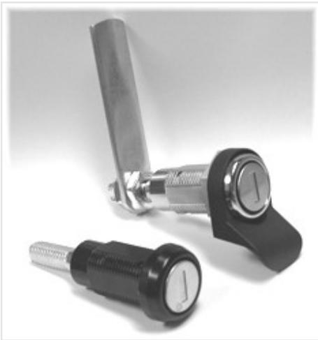
TriMark's 080-0400 CompOne™ Compression Lock combines the compactness of a cam lock with smooth and secure pull-in functionality. Featuring 5mm of compression with a 180° turn of the key, this robust lock is intended for gasketed doors, is fully adjustable, water resistant and easy to install.
